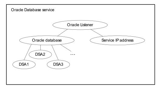
Fig. 4.5: Example of an Oracle database service.
