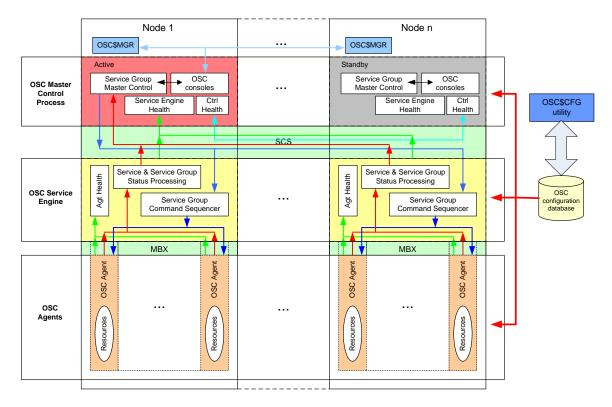
Fig. 4.7: VSI OpenVMS ServiceControl software architecture
