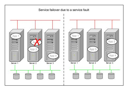
Fig. 4.2: Service failover due to an unrecoverable service failure.
