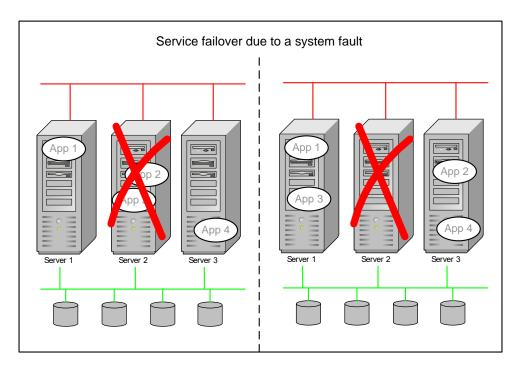
Fig. 4.3: Service failover due to a system failure.
