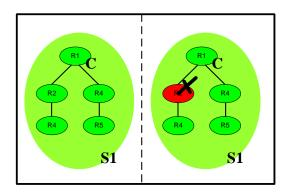
When resource R2 fails, OSC calls the clean action routine. Since R2 is non-critical, fault propagation is not initiated and the service group is not marked faulted. Thus, the resource fault does not cause a service group shutdown and the resource tree is not taken offline.
