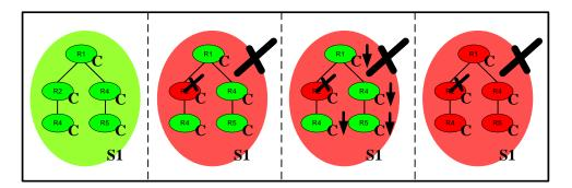
When resource R2 fails, OSC calls the clean action routine and the fault condition is propagated up the dependency tree to service S1. The fault bit in the status field of S1 is set and the fault condition is propagated to the service group. OSC detects that the service group has failed (the service group contains no other services) and shuts down the service
