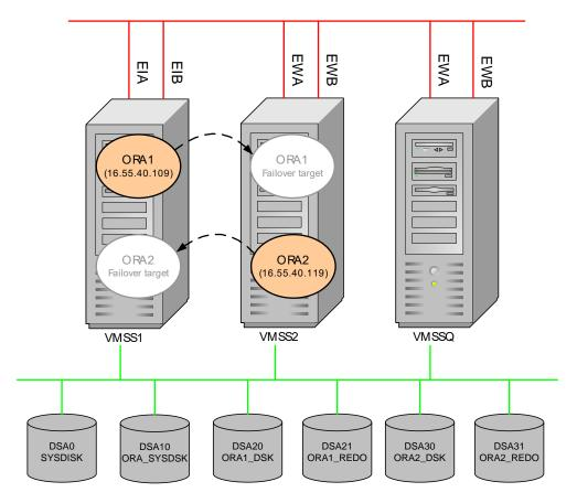
Fig. 8.1:Setup of a three node OpenVMS cluster consisting of node VMSS1, VMSS2 and<br/>VMSQ. OSC will be used to manage the Oracle 10 databases ORA and ORA2.
