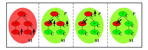
OSC calls the clean action routine for resource R2. Since this resource is non-critical, the fault condition is not propagated up to the service and service group level. Resource R2 is a non-critical resource. Thus, the ONLINE transaction continues to start the service group. After the transaction has completed the final status of service S1 and its parent service group will be ONLINE|PARTIAL.
