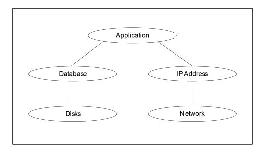
Fig. 4.4: Resource dependency example of an application that accesses a database and uses an IP-interface for inter-process communication.
