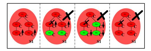
OSC calls the clean action routine for resource R2 and the fault condition is propagated up to the service and service group level. Resource R2 is a critical resource. Thus, the service group is taken offline and failed over to another node in the OSC cluster if the service group is defined as a **Failover** or **MultiInstance** service group.
