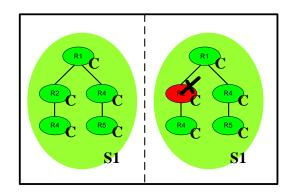
If resource R2 fails, OSC calls the clean action routine. R2 is a critical resource but fault propagation is disabled. Thus, the fault condition is not propagated up to the service and service group level, and the resource fault does not cause a service group shutdown and the resource tree is not taken offline.
