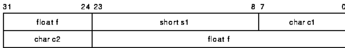
Figure 4.1. VAX Structure Alignment
