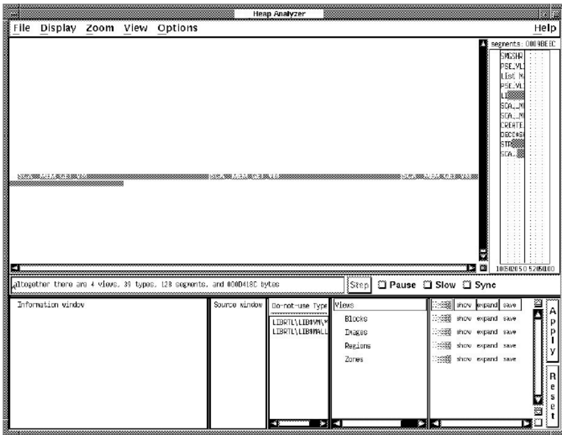
Figure 12.12. Incrementing Memory Allocation Indicates a Memory Leak
