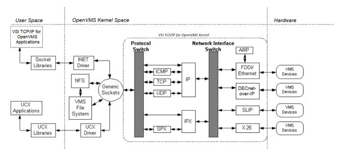
VSI TCP/IP interacts directly with the OpenVMS Operating System. Generic sockets pass requests to the protocol switch, that differentiates between requests for IP use and for other support facilities. Requests are then sent through the network interface switch, which identifies the device for which the request is bound. When a request is received from a device, the steps occur in reverse.
